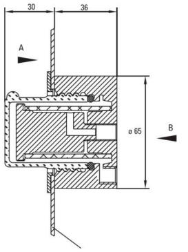
bore-hole in frontpanel ø 50
